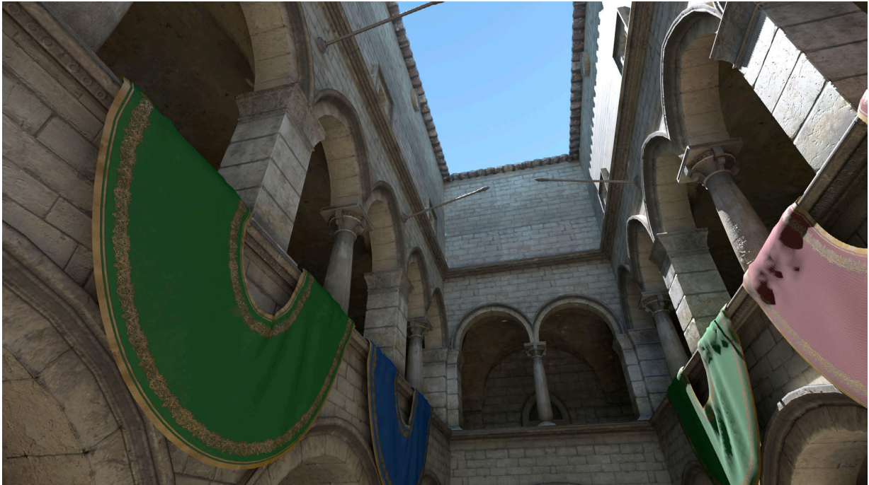
(a) Real-time render using indirect illumination from a baked lightmap. The lightmap uses the Ambient Dice cosine-lobe variant for both diffuse and specular (Section 8.3).
